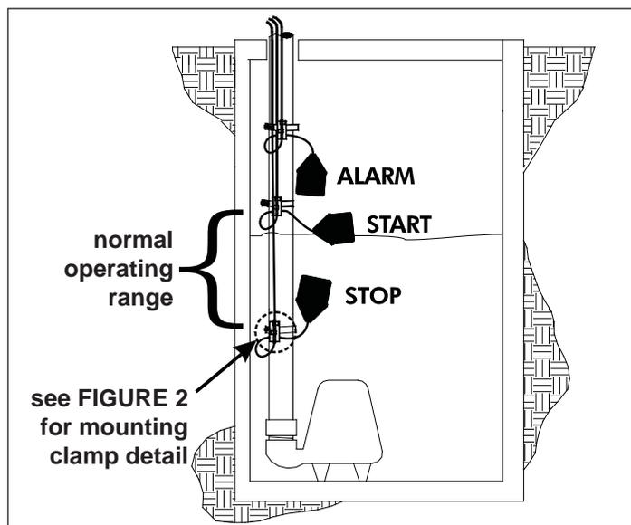
**FIGURE 1 - Three float simplex -
